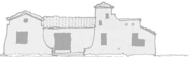
Loggia partially filled in, window dimensions and configurations changed
